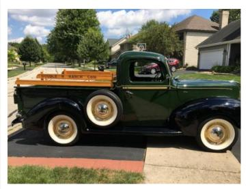
This 1940 Ford 1/2 ton pickup is a full restoration. The engine is a 1951 Mercury flathead, 3 speed transmission, Columbia two speed rear end. Frame is powder coated along with many suspension parts. New wire harness and many other items. Have all the records of the restoration and list of parts. Asking \$40,000. Contact Ron Steck at 630-777-4001.
