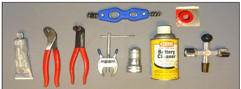
BATTERY TOOLS (Left to Right): Dielectric Grease, Square-jaw Battery Pliers, Battery Terminal Spreader Tool, Battery Terminal Puller, Battery Terminal and Post Wire Brush Tool, Battery Acid Cleaner/Neutralizer, and Battery Terminal & Post Reamer. (Top): Another style of Battery Terminal & Post Wire Brush, and Battery Post Anti-Corrosion Pads.
